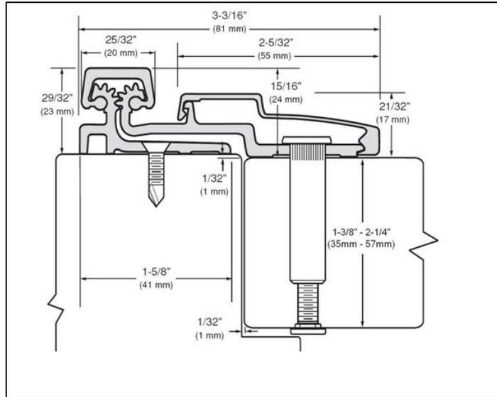
HD210 is an Aluminum Continuous Geared Full Surface Hinge that provides a 1/32" door inset. It can be used with any standard frame without hinge preps, and either with or without reinforcements depending on door weight. The frame face must have a flat surface at least 1-5/8" wide. Clearance between the hinge edge of the door and the frame rabbet is 1/32" (1mm). "HD" models have additional bearings and frame fasteners for heavy-duty application.
