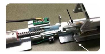
• Install (2) screws with allen wrench provided to secure the motor moun to the baserail.
