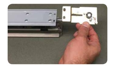
• Remove (2) screws from back of the push pad.
