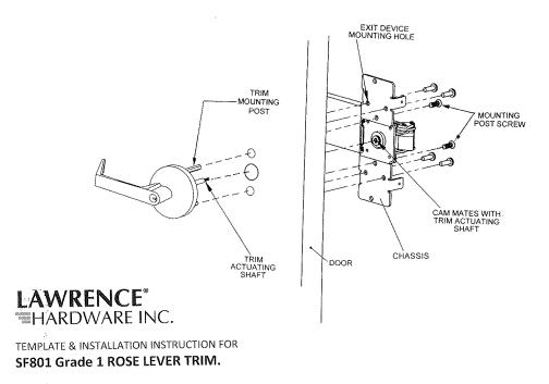
Not to Scale The use of non-clutching impact drivers to install this hardware will automatically void the warranty.
