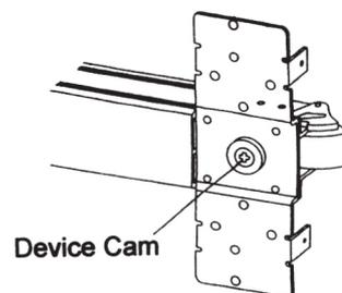
INSERT TRIM ACTUATING SHAFT INTO DEVICE CAM " + "
