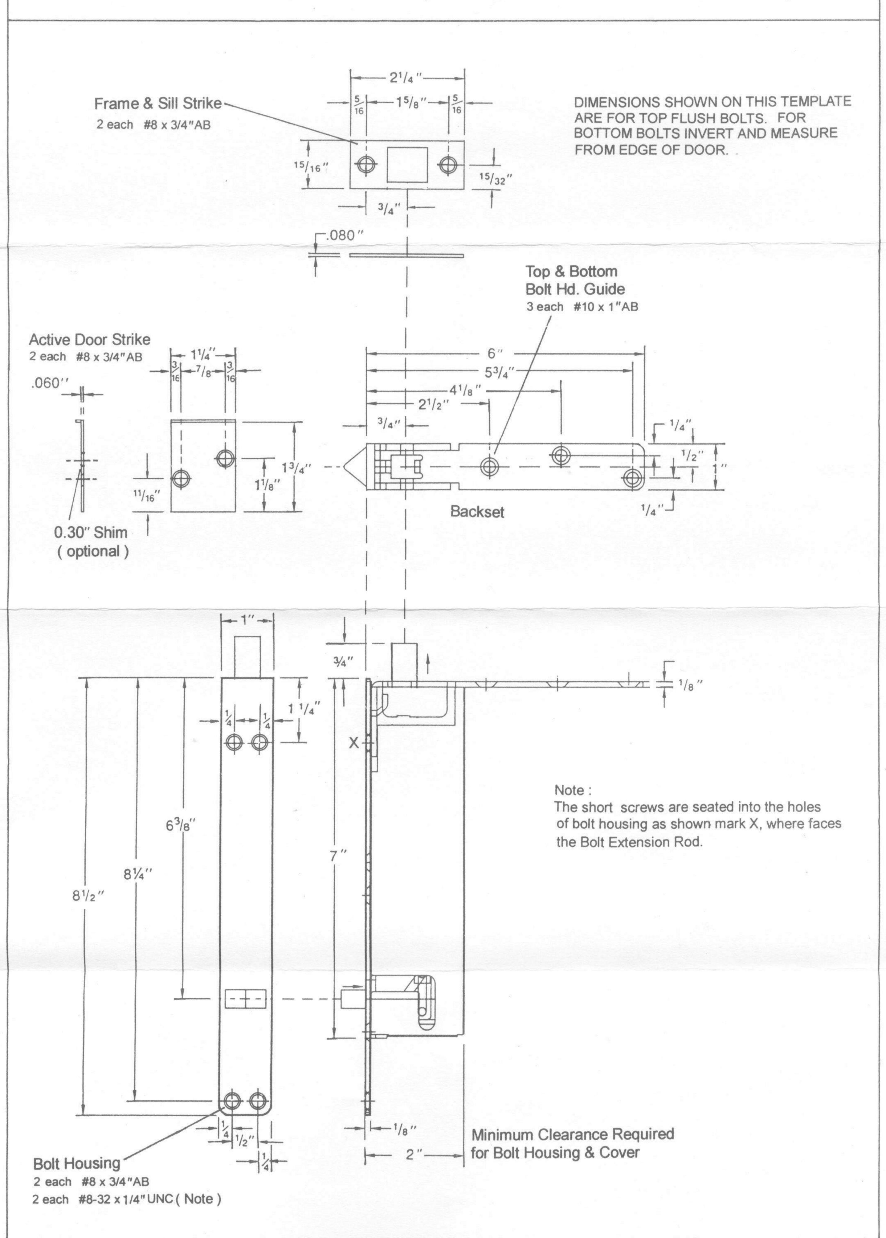
SCREW DETAILS: #8-32 x 1/4" UNC - flat countersunk head machine screw, total 2 pcs.
