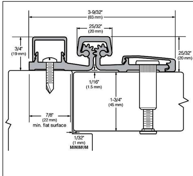
HD157 is an Aluminum Continuous Geared Full Surface Hinge that provides a 1/16" door inset. It can be used with any standard frame without hinge preps, and either with or without reinforcements depending on door weight. The frame face must have a flat surface at least 7/8" wide. Clearance between the hinge edge of the door and the frame rabbet may be from 1/32" to 1" (0.8 – 25.4mm). "HD" models have additional bearings and frame fasteners for heavy-duty application.
